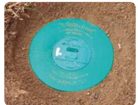
Picture 1: Shows Sentricon soil-cover sitting flush with the soil surface, also shows station number.
