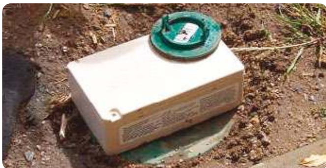
Picture 9: SMAG (Soil Mounted Above-Ground station)
