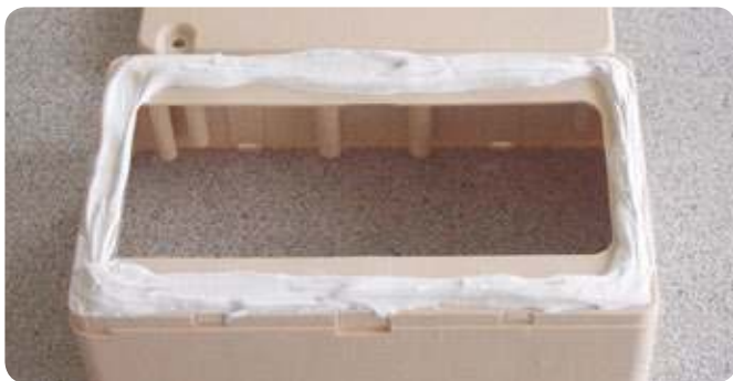
Picture 8: No-More Gaps sealant applied to the base of a Sentricon AG station
