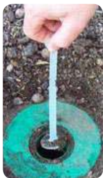
Picture 7: Extractor that has been modified to clean out debris from inside IG stations in case no other tool is available.
