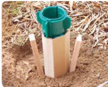
Picture 3: IG stations should be installed with at least 2 external monitoring devices. To prevent soil from falling into the station during install wrapping it in cardboard can be beneficial.
