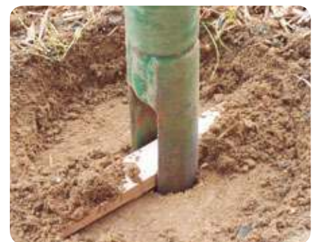
Picture 2: Shows MD in auger channel, a technique used to create a flat base for the Sentricon soil-cover. Can be used to remove lawn thatch, gravel or mulch.
