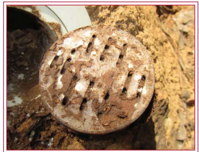
Nasutitermes feeding in in-ground canister.
