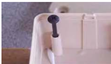
Photo 2. Internal screws hold the station to the mounting surface.
